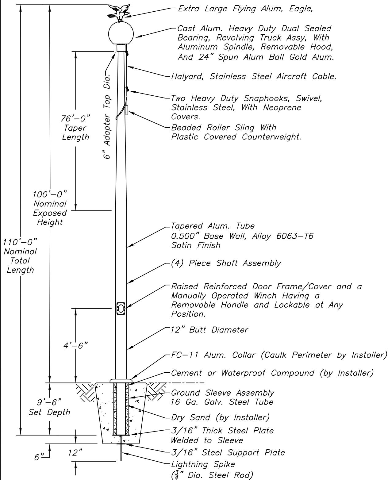
NOTE: FOUNDATION DESIGN NOT INCLUDED. FOUNDATION DIMENSIONS SHOULD BE DETERMINED BY A QUALIFIED ENGINEER FAMILIAR WITH SITE SOIL CONDITIONS.
